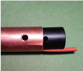
You will need to insert the bushing with the rubber cord into the end of the shedding device. The rubber cord serves two purposes: It allows for a snug fit of the bushing and it allows you to remove the bushing to put on another loom. Line up the bushing hole with the shedding device hole and push in until the two holes are in the same position.
